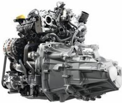
The all-new TCe 110 has variable valve timing, variable displacement oil pump, and use of multiple high-efficient materials combine to help boost performance and reduce fuel consumption. The integrated exhaust manifold, particle filter, and central injector help reduce CO<sub>2</sub> emissions.
