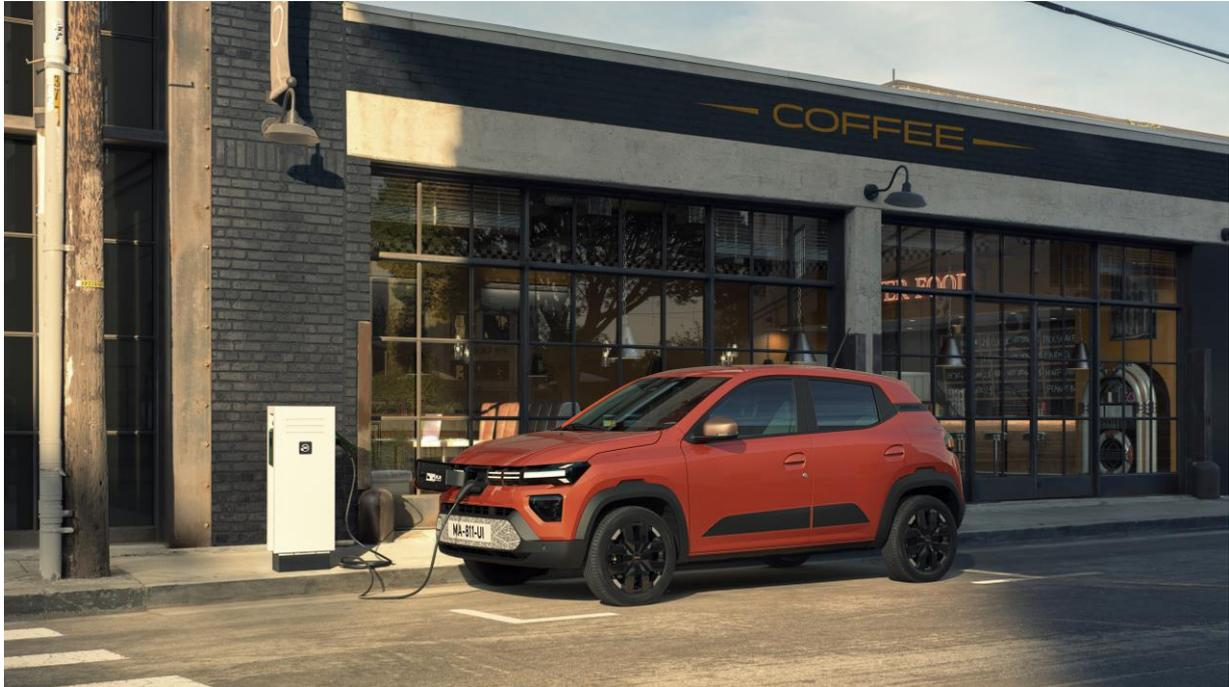
**How about a barbecue with your new Spring?** More practical than ever before, the New Dacia Spring now features a bi-directional V2L (vehicle-to-load) charger so it can be used as an energy source to power electrical devices. A specific adapter that plugs into the car's charging connector, located under the grille, acts as a traditional 220V/16A socket.
